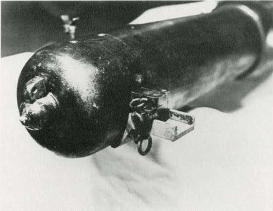
FIGURE 2. This photograph shows the right side of the breech. The two metal wedges rest one atop the other in the tray. The lower wedge had a handle which protruded parallel to the axis of the barrel. By pushing it away from the barrel, it caused the wedges to work against each other, loosen the interior breech mechanism, and finally slide out into the tray. The rings probably had chains on them which kept the wedges from being lost from the barrel.
