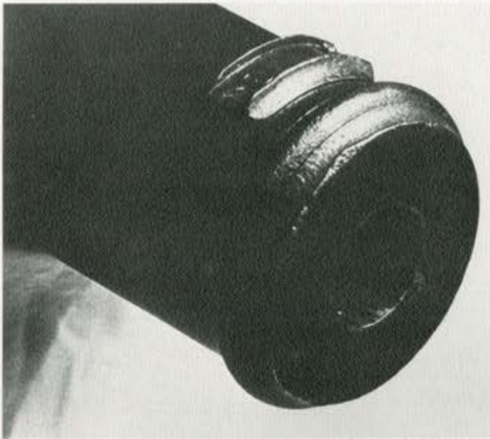
FIGURE 5. This close-up photograph of the muzzle shows the rifling (visible at the edge of the shadows at the lower right of the bore).
